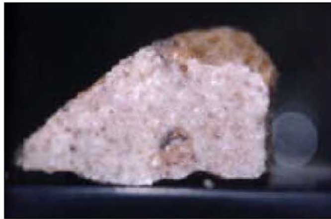
Fig. VI-40. BaSO_4 layers formed on sandstone.
